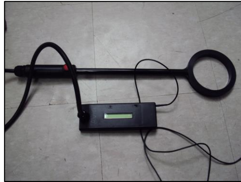
Wand used to read AVID Chips
