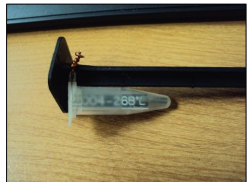
AVID Chip Attached to Ground Stake
