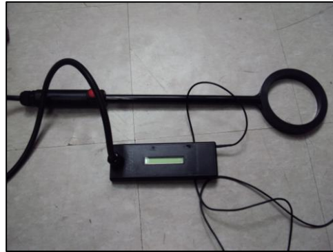
Wand used to read AVID Chips
