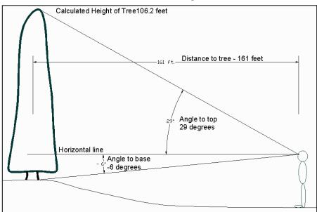
In order to determine these three pieces of information, you will need to use a clinometer in conjunction with an electronic range finder or tape measure. The clinometer can determine the angles, the electronic range finder or tape measure can determine the distance.
